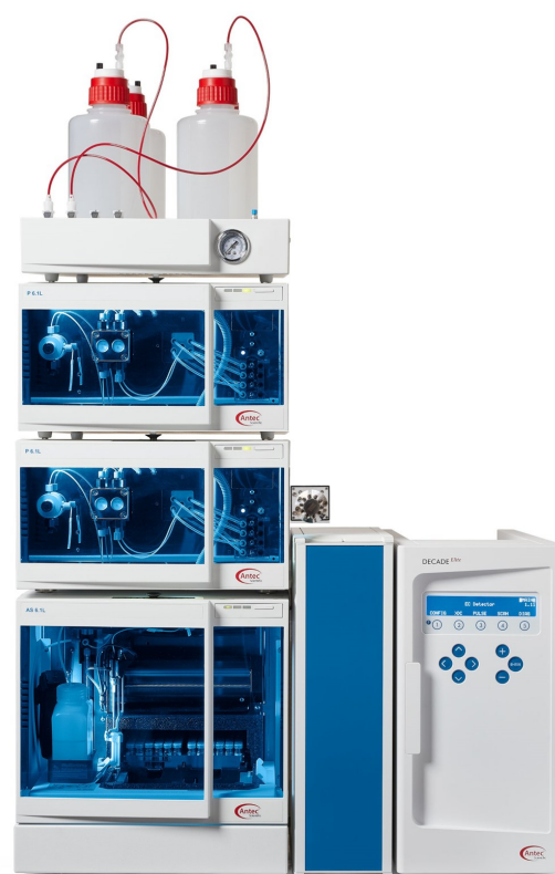
Figure 1. ALEXYS High-throughput Carbohydrate Analyzer.
